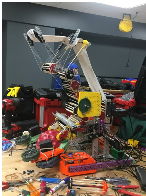
Figure 111: Improved V1 Hood with Increased Gear Ratio and less trusses
