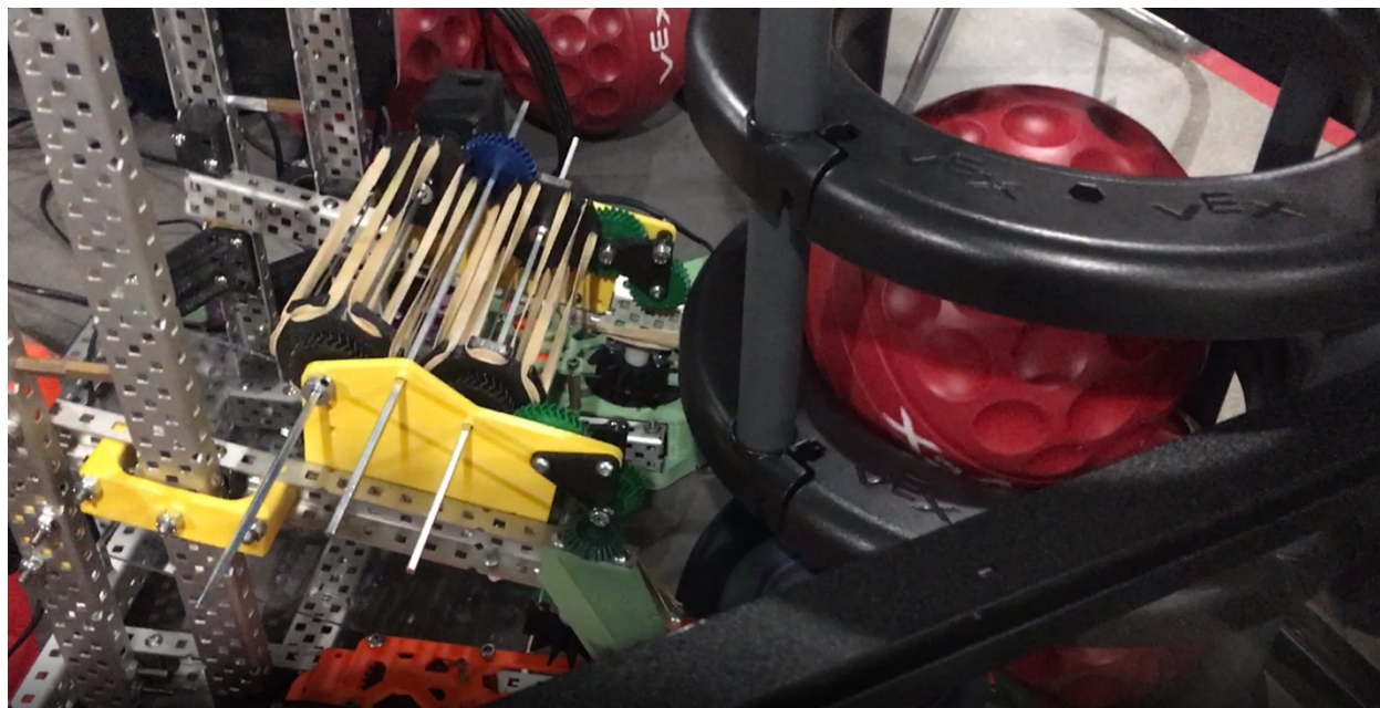
Figure 99: Testing the first prototype of the lower rollers in real life
