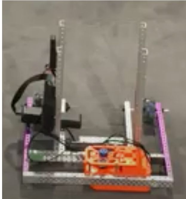
Figure 65: Single V3 swerve module attached to chassis for testing
