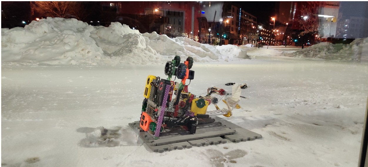
Figure 4: Robot out in the snow to cool down overheating swerve motors
