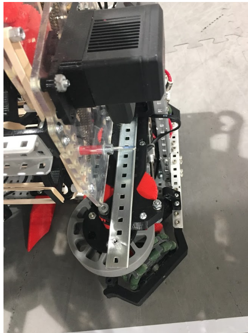
Figure 90: V3 Intakes retracted linearly to be within frame
