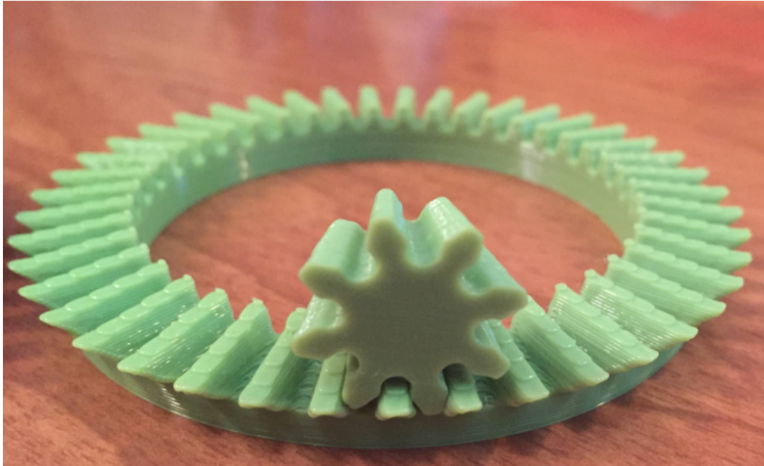
Figure 53: V2 bevel gears with undercutting
