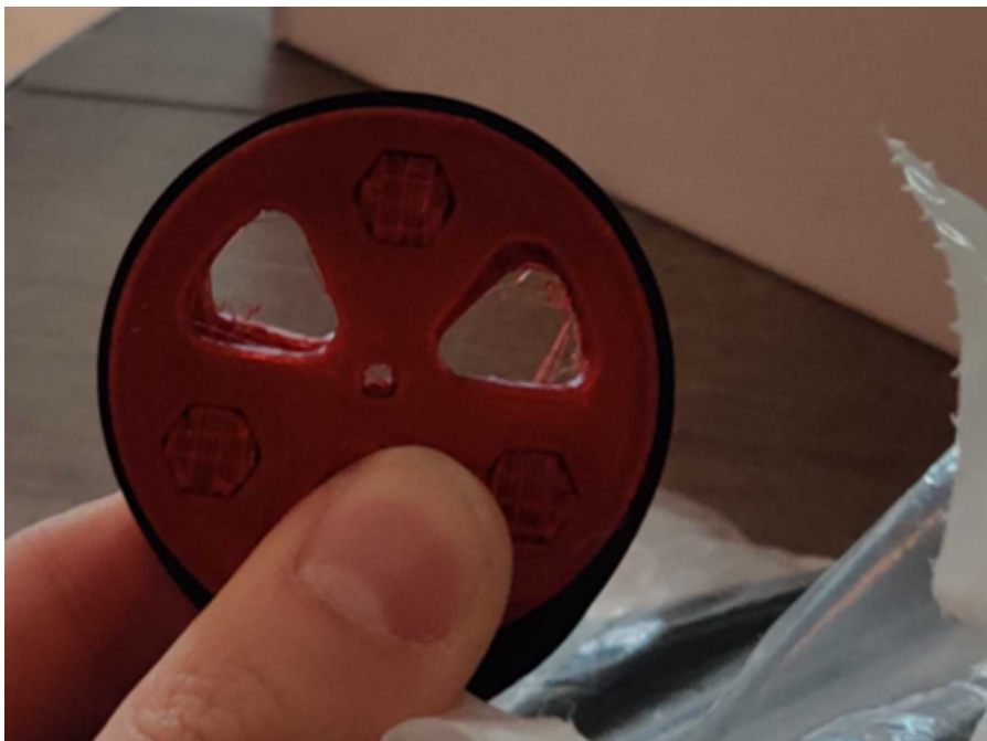
Figure 63: 3D printed wheel with neoprene tread
