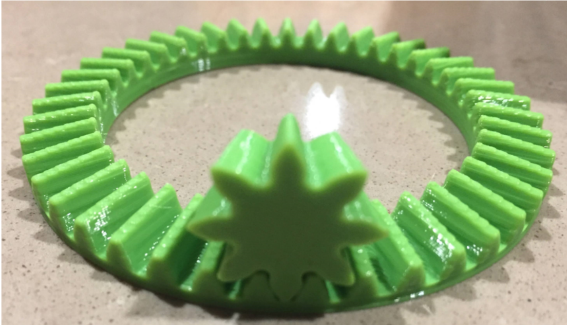
Figure 54: V3 bevel gears with tapering
