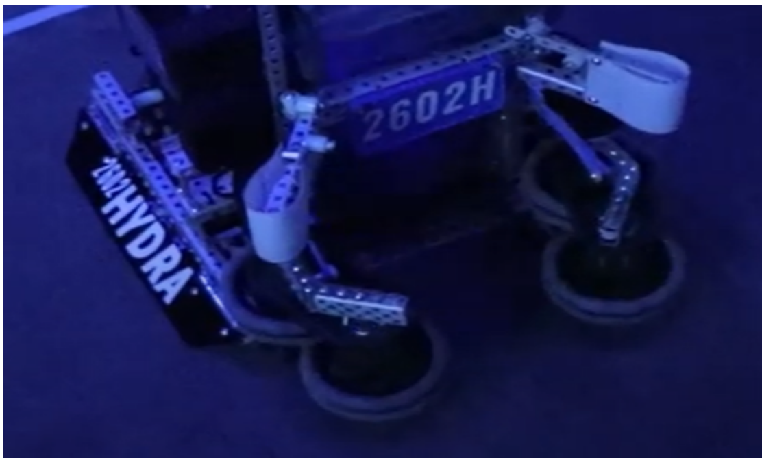
Figure 82: An example of an omni wheeled intake employed by VEX team 2602H
